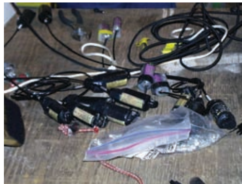
Figure 7. A radiotransmitter is about the size of D cell battery (about 3 to 4 ounces) and is attached to a 14-inch antenna. Radiotransmitters send specific radio signals for tracking individual turkeys.
